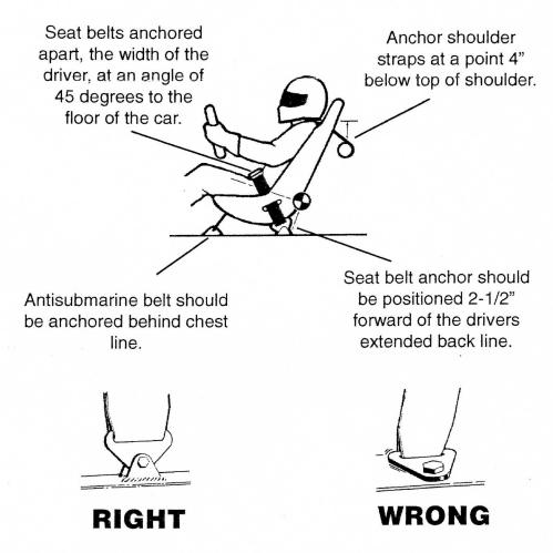
Mounting brackets should be installed at an angle that is compatible with the direction of pull on the webbing under full load.
